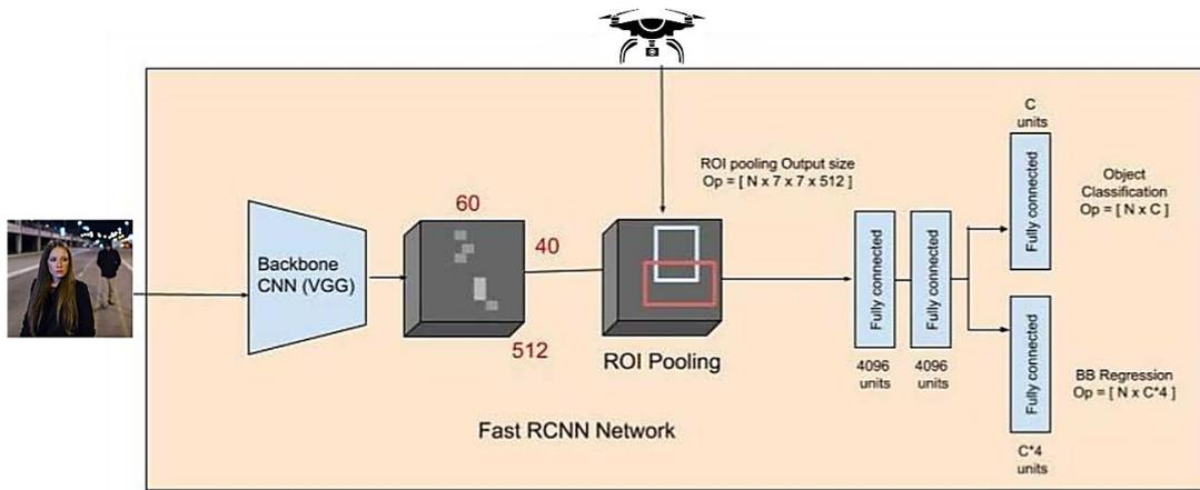
Fig. 1. Fast R-CNN pipeline
